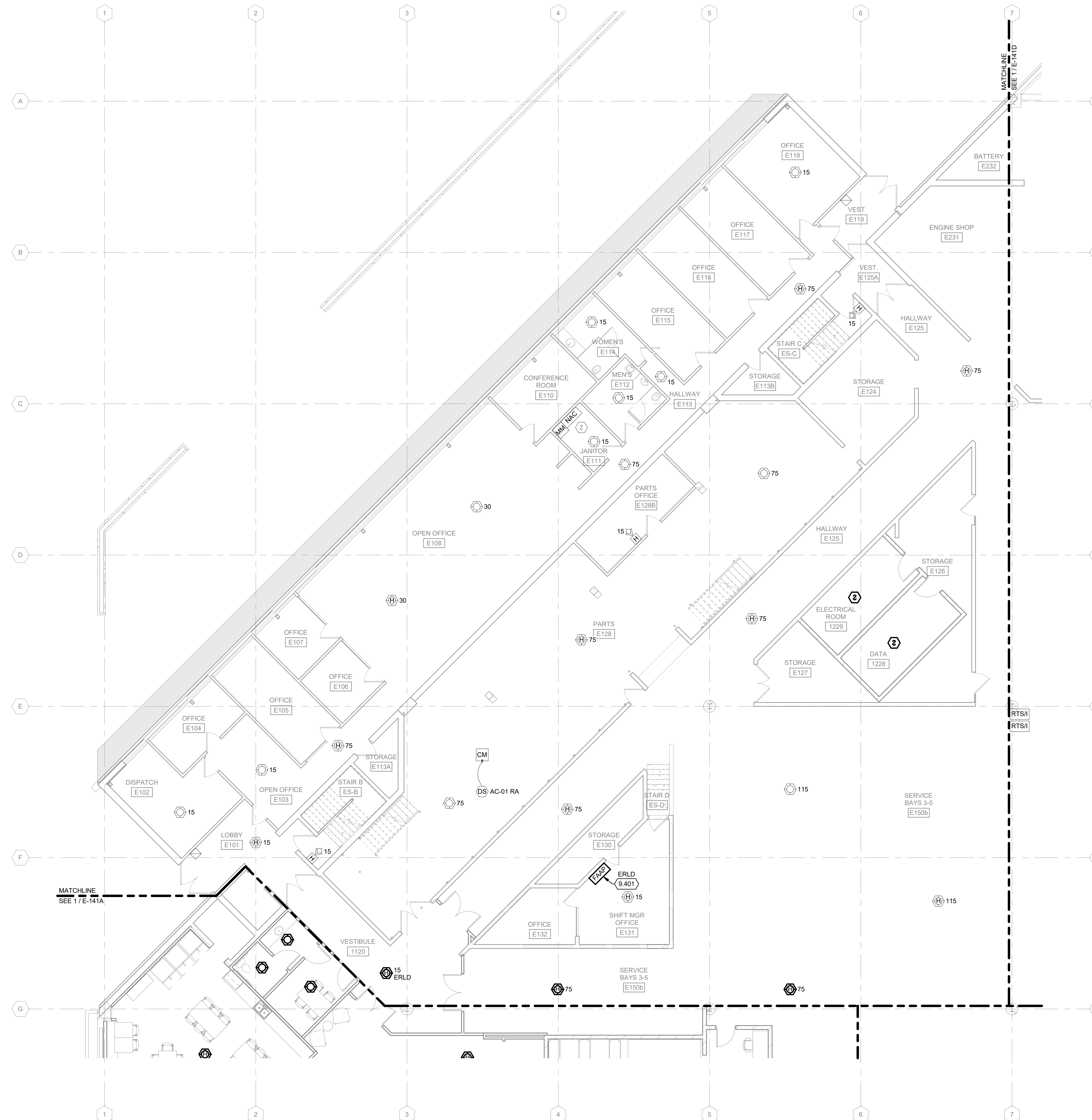
1 FIRST FLOOR FIRE ALARM PLAN - AREA B 1/8" = 1'-0"
